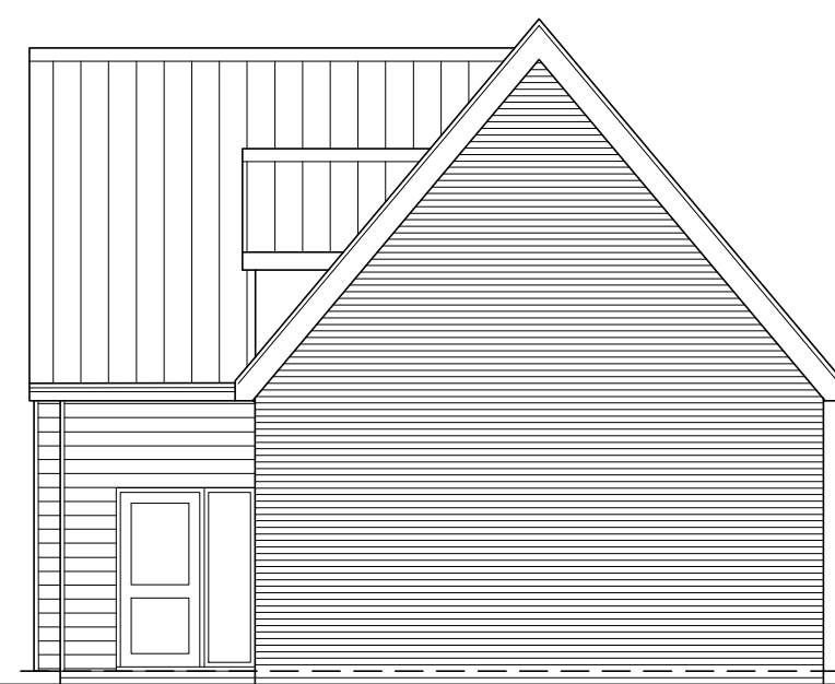
Side Elevation - South East 1:100
