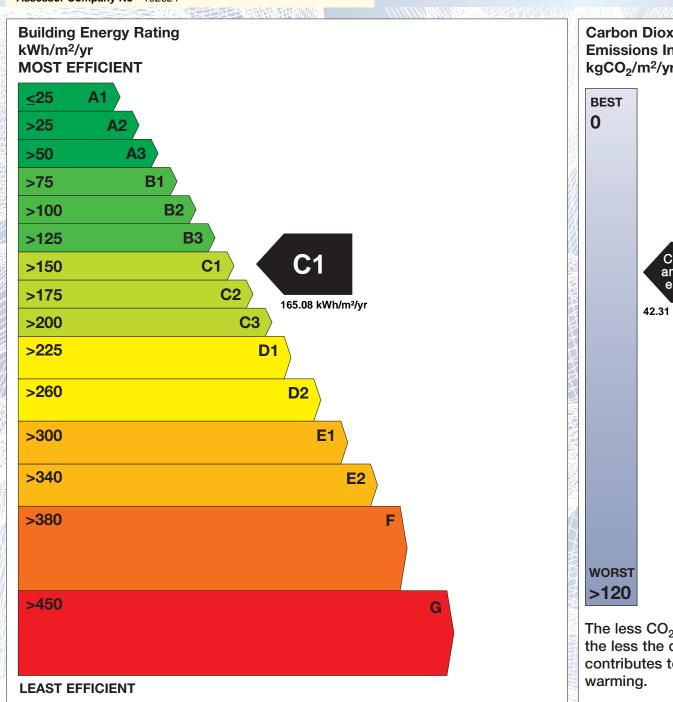
Carbon Dioxide (CO<sub>2</sub>) **Emissions Indicator** kgCO<sub>2</sub>/m<sup>2</sup>/yr Calculated annual CO2 emissions 42.31 kgCO<sub>2</sub>/m<sup>2</sup>/yr The less CO<sub>2</sub> produced, the less the dwelling contributes to global
